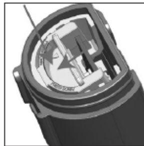
Fig. 4: Push down to lock
