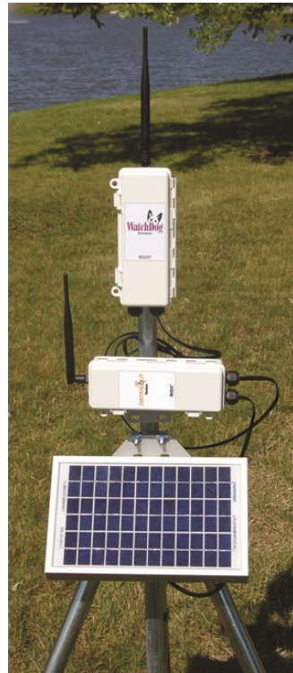
Figure 4. Retriever and DataScout setup with solar panel
