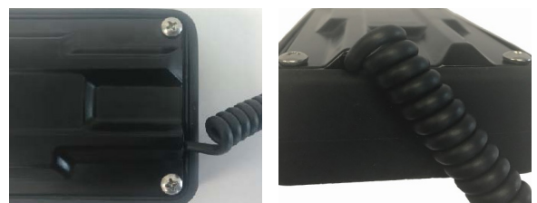
Sensor cable fed through the slot
