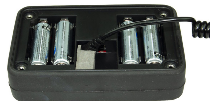
Sensor cable, batteries and foam insert
