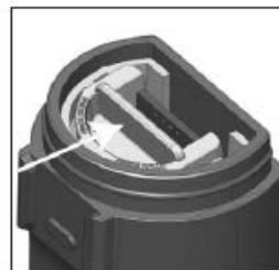
Fig. 2: Push to unlock
